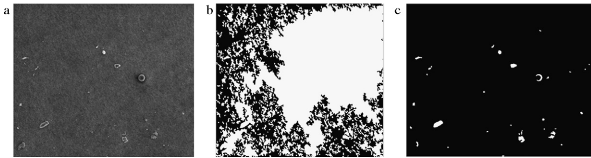
Fig. 6. Comparison of SVM predicted algorithm with other methods: (a) SEM image of collected particles on filter paper, (b) SVM predicted method (Kapur thresholding) output, (c) Otsu thresholding output.
